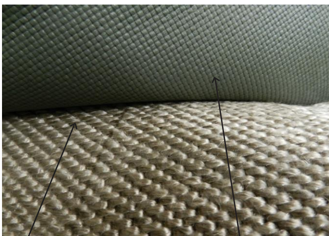
PTFE Corrosion / Gas Barrier Weight: 13.5 oz/yd 2 (458 g/m 2 ) Thickness: 0.009" (0.23mm) Tensile Strength: 25 lb/in (223 N/50mm)
